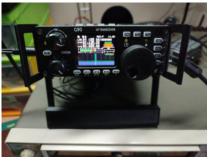
Figure: Xiegu G90 is an example of zero-IF SDR HF transceiver
